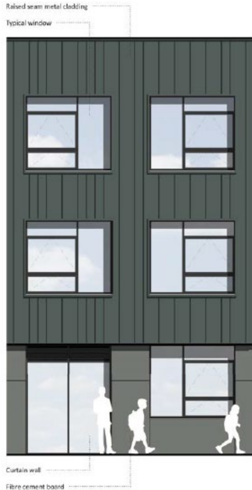
Typical Elevation Bay Study
